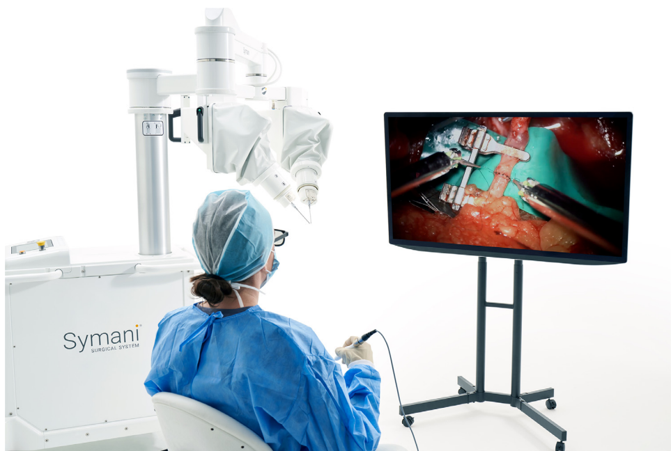
Figure 5. The robotic microsurgery platform Symani. Note the microneedle holder and forceps attached to the robotic wrist in which the master (surgeon) controls from the console. Image courtesy of Medical Microinstruments, Inc.
